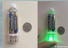
Figure 5: Fishtek Marine® UltraBright ProGlow submersible green LEDs, (λ = 520nm, 0.7 lumen) with quarter for scale.
