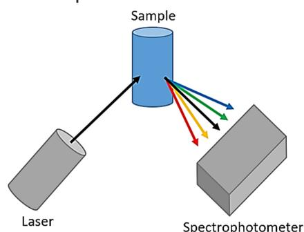
Figure 1 A diagram showing the process of Raman Spectroscopy. Diagram produced by Emily Blacklock.
