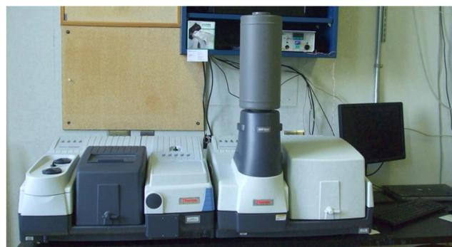
Figure 2 The Nicolet NXR 9650 FT-Raman Spectrometer. Photograph by Michel Johnson.
