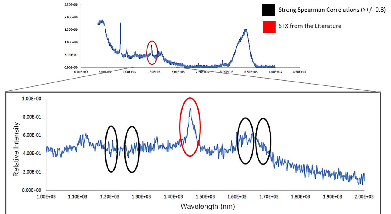
Figure 3 The raman spectra from the hemolymph of a *Homarus americanus*, with a STX concentration of 150.4 µg/100g STXeq, where significant peaks are circled.
